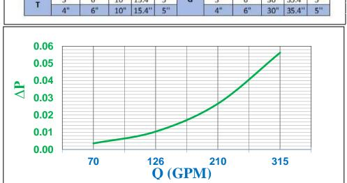
Flow data for a 2" Style "RS" short with a process fluid of 500 cps. Perforated element with 10 mesh 1900 micron overscreen.
